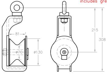
REF OCN1 for NYLON SHEAVE REF OCC1 for CAST IRON SHEAVE
