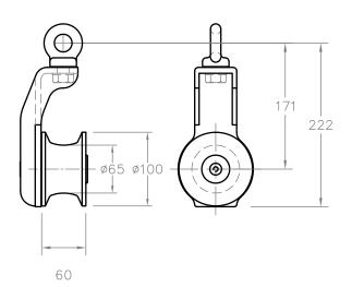
1 TON OPEN SIDED POTTING BLOCK with nylon replaceable sheave.
