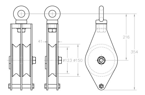
2 TON GILSEN BLOCK WITH BECKET SINGLE SHEAVE ...... WT. 8.8 KG. DOUBLE SHEAVE ...... WT. 14.2 KG.
